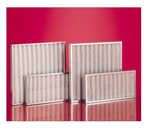
AmerTex F30 is a strong, multi-layered media, folded into uniformly shaped pleats to ensure an even dust loading over the surface of the filter which is necessary for high efficiency filtration. AmerTex F30 is classified F5 in accordance with EN 779.
